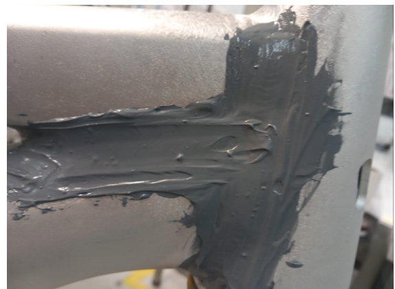
(b) Epoxy putty applied to junction of HT, TT and DT.
