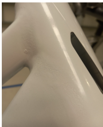
(a) Example of outgassing defect.
