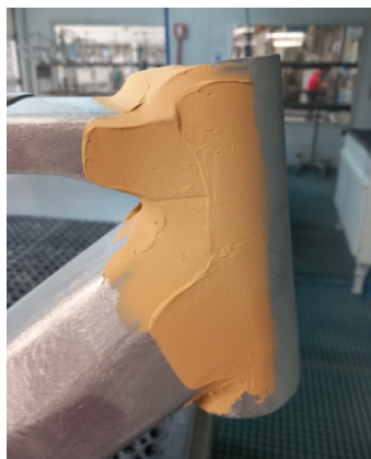
(a) Polyester putty applied to junction of HT, TT and Down Tube (DT).
