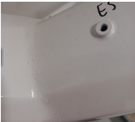
(a) Failure of the 1k primer in the ES putty.
