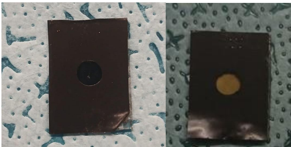
Figure 4.5: MAPbI 3 cell before (left) and after (right) the 583 hour UV-exposure period.
