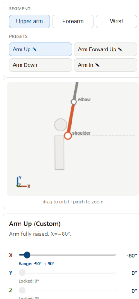
Figure 4.20: Interactive 3D movement visualization in the Rehab Sequence Editor, providing a real-time preview of the limb posture corresponding to the configured joint rotations.
