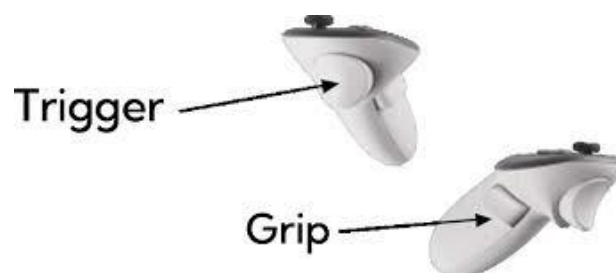
Figure 13: Trigger and Grip Buttons on Meta Quest 3 Controllers [67].
