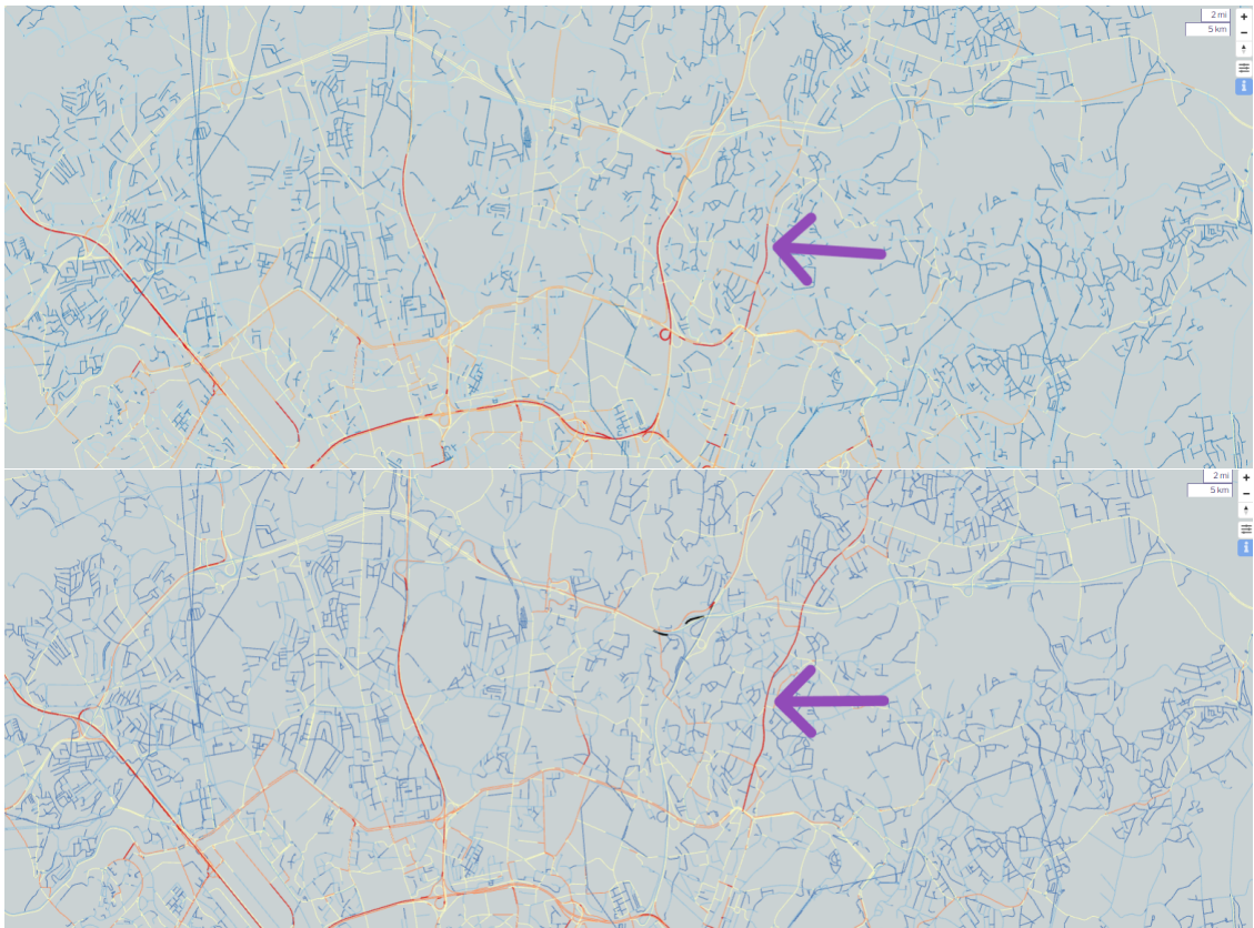
Figure 4.3: Comparison of traffic conditions at peak hour for the baseline scenario (top) and for the scenario with the three selected links closed (bottom)
