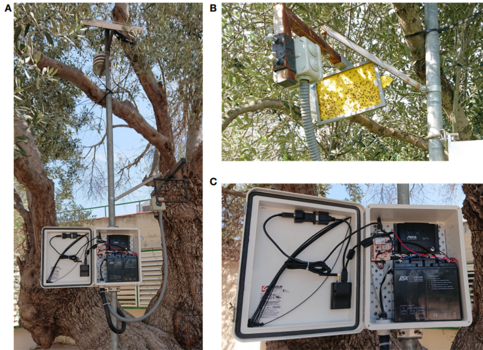
Figure 2.15: Electronic components of the e-trap system (A) E-trap with solar panel, Stevenson screen to protect the temperature and relative humidity sensor, battery and electronics. (B) Camera placed in front of a Rimi® trap. (C) Battery and electronics. [30]
