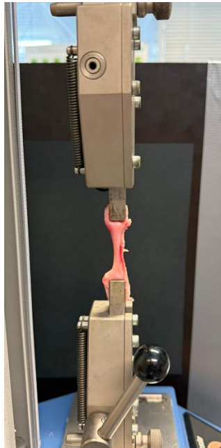
Figure 30 Uniaxial stress test of the vaginal tissue.
