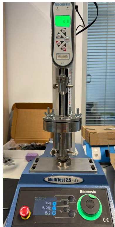
Figure 21 Ball burst machine used to perform ball burst tests.
