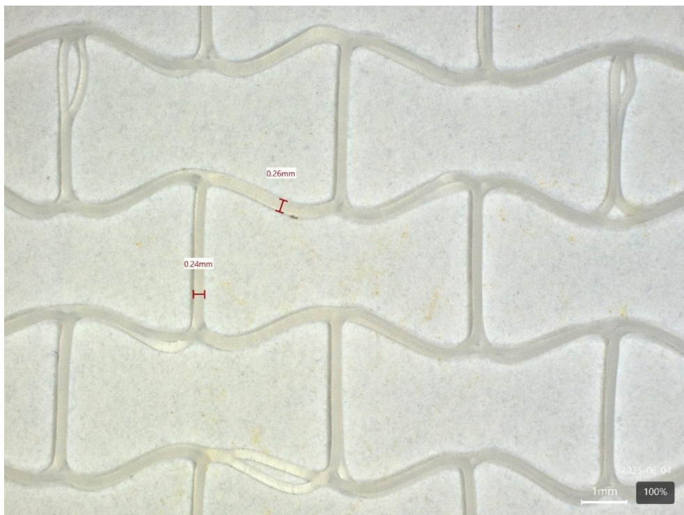
Figure 25 Photograph of the digital microscope view of the re-entrant honeycomb mesh.
