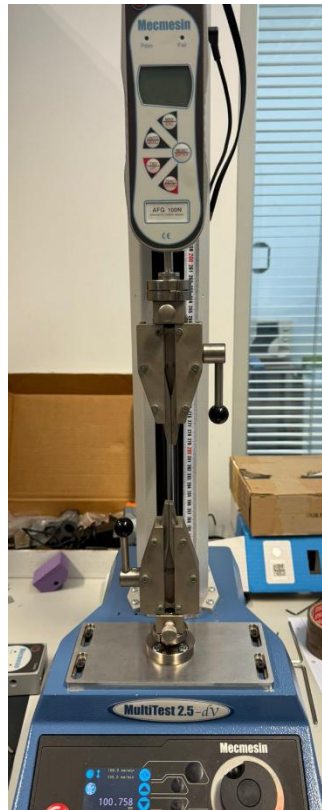
Figure 20 Uniaxial tensile test machine used to perform uniaxial tensile tests.
