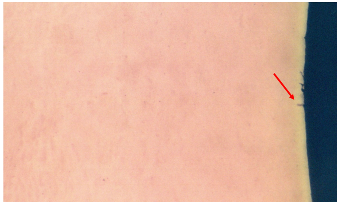
Figure 2.6: Vented water tree 120\ \mu\text{m} long (indicated by the red arrow) approximately 2% of the insulation thickness [52]
