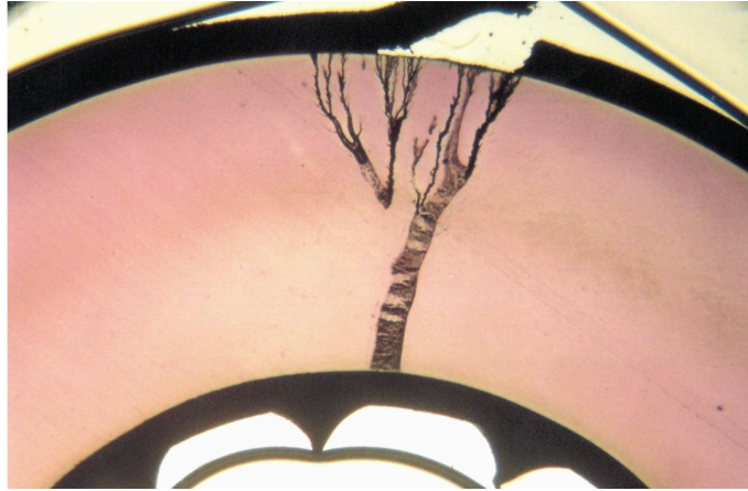
Figure 2.7: Electrical tree directed toward the insulation screen, indicating breakdown initiated from a bow tie tree or from the conductor screen [52]
