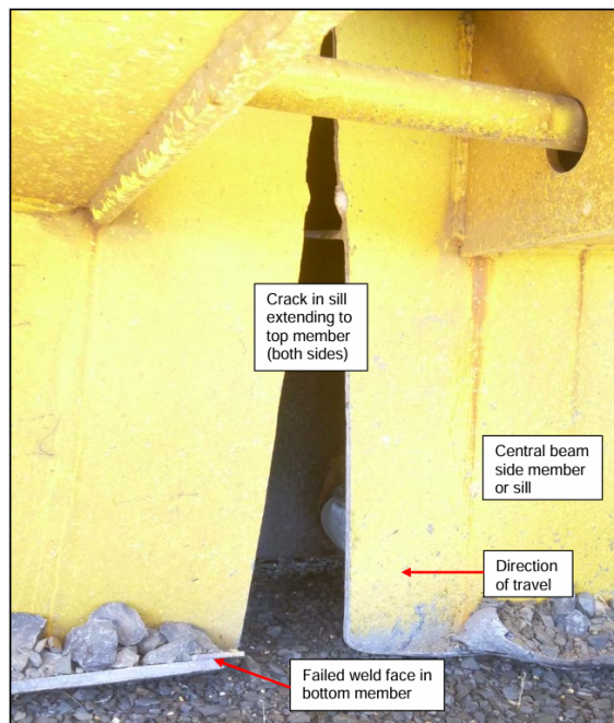
Figure 2.1: Side view of failure in wagon SQDY 00060G [24].
