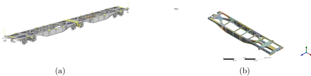
Figure 2.10: Example of Sggrss wagon (a) and generated model in Ansys (b) [41].
