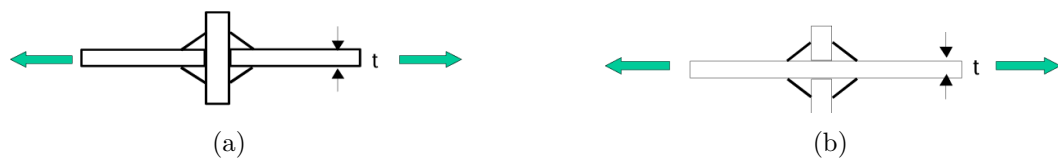
Figure 4.16: Schematic of a load-carrying (a) and a non-load carrying (b) welded connection (adapted from Dong et al. [13]).
