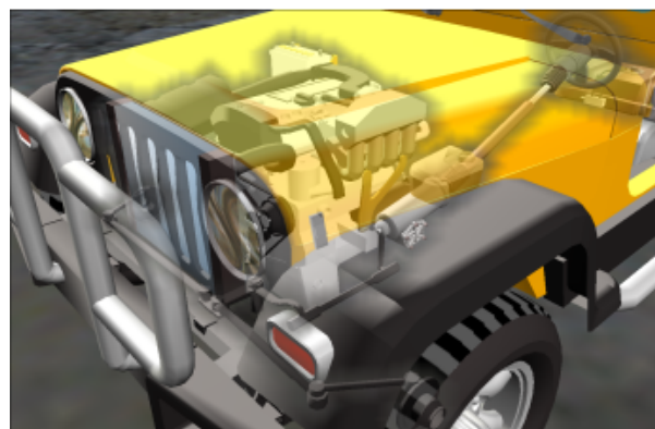
(b) Dynamic-transparency rendering for occlusion management, revealing hidden structures while preserving spatial context. Taken from Elmqvist, As-sarsson, and Tsigas [21].
