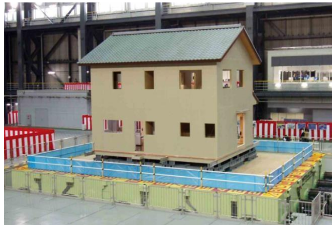
Figura 2 - Mesa sísmica (Fonte: National Research Institute for Earth Science and Disaster Resoalience (NIED))
