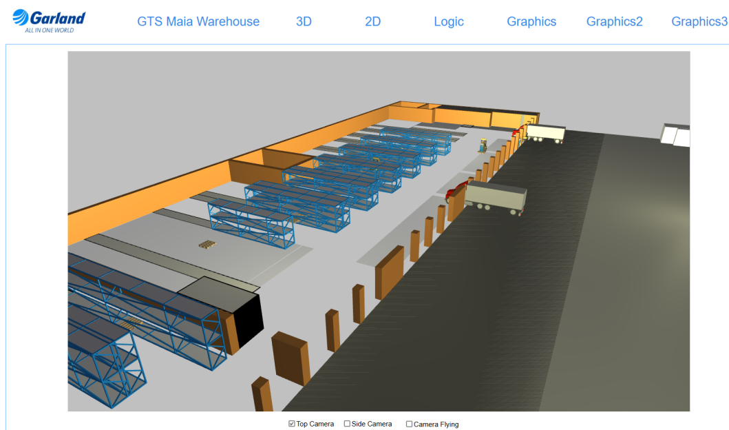
Figure J.2: 3D view of the GTS Maia warehouse simulation model in AnyLogic , showing the physical layout, racking structures, dock doors, and truck and forklift agents during the baseline simulation run.
