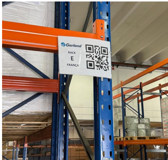
Figure C.5: QR codes identifying individual rack positions
