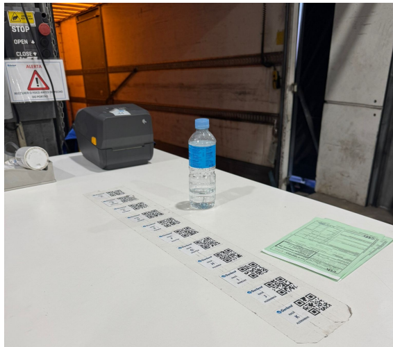
Figure C.6: Barcode labels used on warehouse worktables to register cargo storage locations in the WMS
