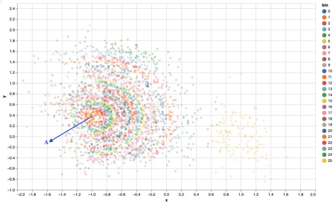
Figure 10.1: Sampling of an audio unit within a two-dimensional t-SNE projection of the RAVE latent space using the k -NN binning strategy. Discrete latent units are represented as points, with the reference unit (A) indicated by a blue arrow. The color gradient signifies the organization of units into discrete “bins” based on spatial proximity, where each bin corresponds to a specific value of the closeness parameter C .
