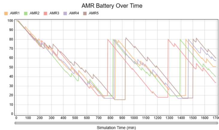
Figure 4.5: Battery level evolution of the AMR fleet over a representative run.
