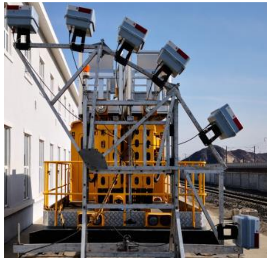
Figure 33 - Air-coupled radar (Lei et al. , 2023)
