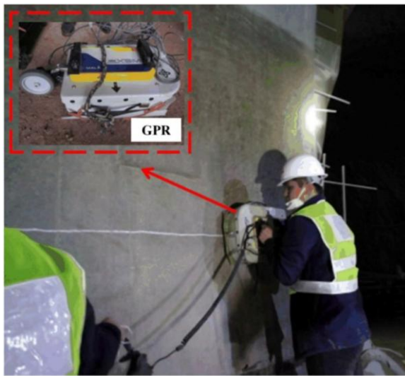
Figure 32 - Ground-coupled radar (Geng, Ye e Wang, 2022)
