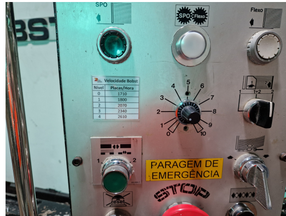
Figure 23: Press speed conversion reference installed next to the speed dial.
