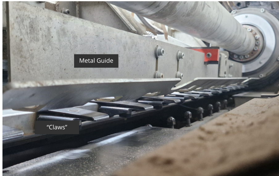
Figure 19: Metal guide at the claw entry point of the Bobst press introducer.
