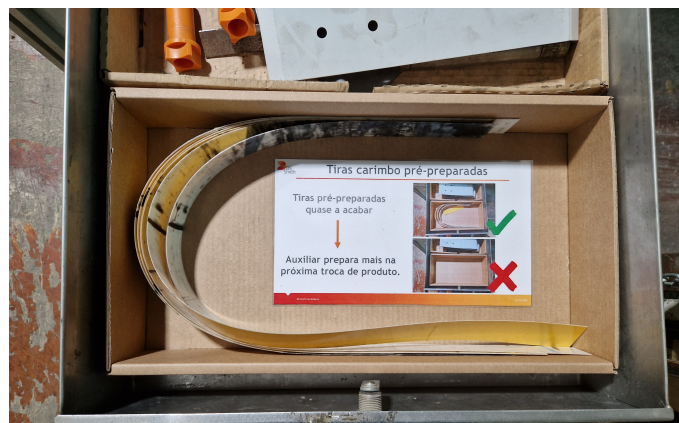
Figure 21: Drawer with pre-prepared plastic strips for counter plate adjustments.
