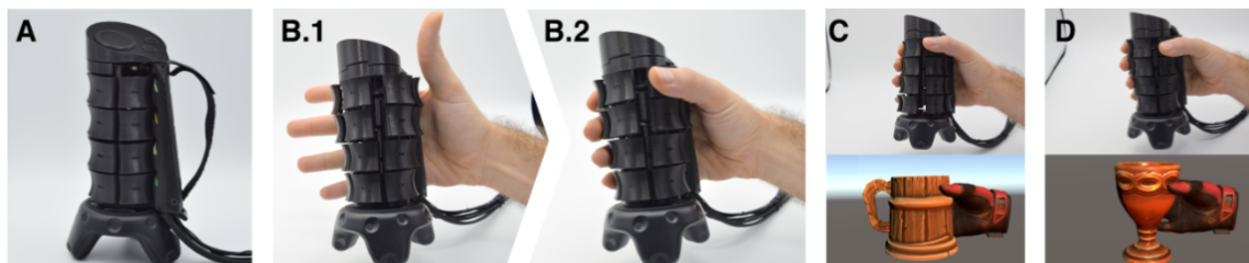
Figure 2.14: X-Rings (A) is a 360° shape display designed to support grasping. The device is hand-mounted (B.1), allowing the fingers to grasp and release rendered objects freely (B.2). Four expanding layers enable rendering of many virtual objects, such as a tankard (C) and goblet (D) [27]
