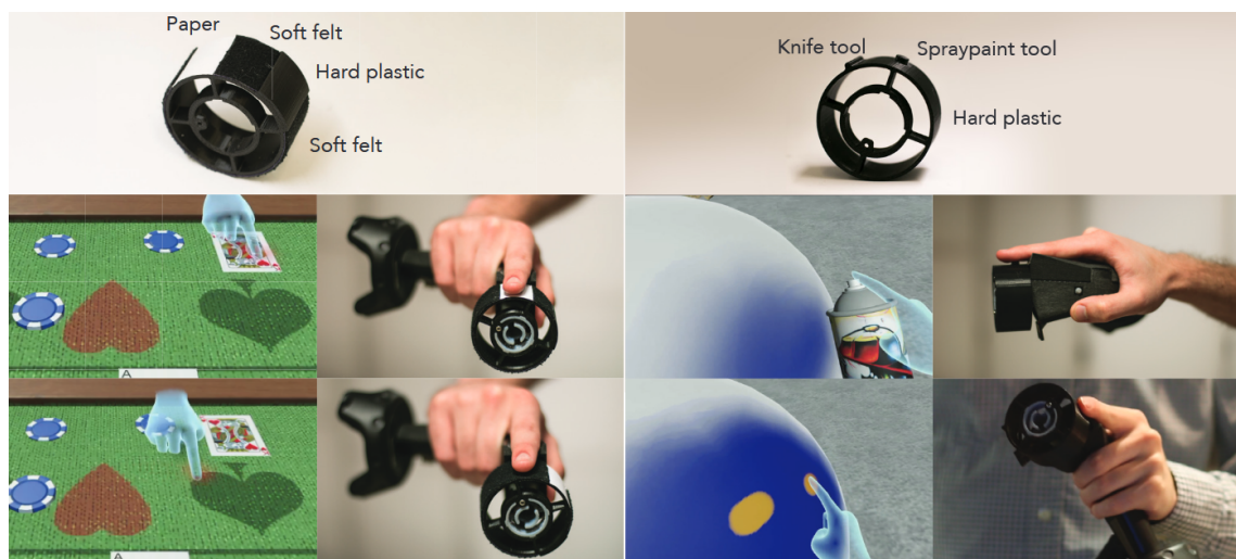
Figure 2.21: Haptic Revolver with two different cylinders[72]
