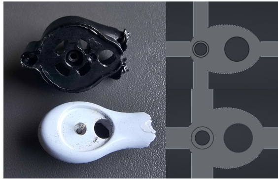
Figure 3.2: The two different fan mounts and their 3D model equivalent
