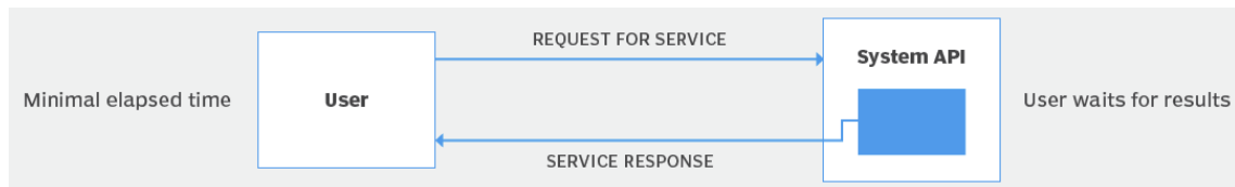
Figure 2.3: Synchronous API call, illustrating the communication between a user and a system API , where the user waits for the response before proceeding [61].
