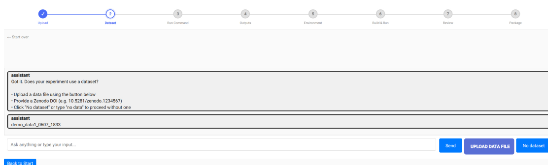
Figure 4.5: The dataset stage of the packaging workflow. The stage tracker shows the position in the workflow, the assistant message states the available options, and the same decision can be made through the buttons or through the chat input.
