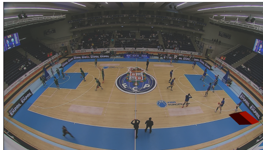
(c) With Distortion Applied. Virtual elements rendered with simulated radial distortion, exhibiting more geometrical alignment between the virtual world and the real one.
