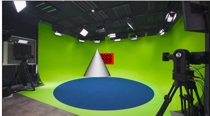
Figure 3.5: Illustration of visual misalignment despite correct center-shift calibration. Although the virtual cone appears offset from the center of the target, this is due to changes in the camera's pan and tilt angles. The center-shift values remain correct; the apparent offset is a result of perspective shift introduced by the camera orientation. This highlights the importance of resetting pan, tilt, and roll to zero when verifying center-shift calibration. 1
