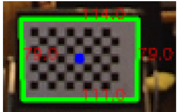
(d) Zoomed edge detection result. Detailed view of the extracted geometry, confirming detected corners and displaying edge lengths (in pixels).
