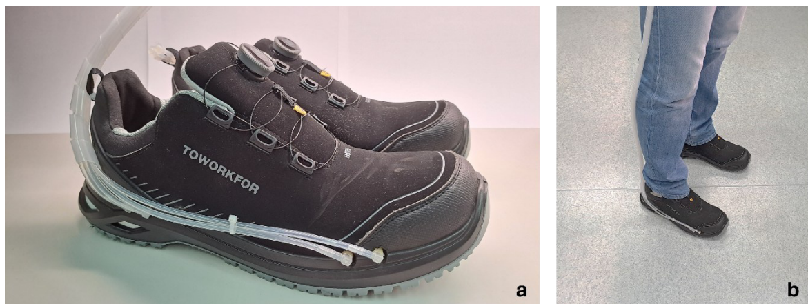
Figure 3.11 – Safety shoe (TOWORKFOR®, X-506) used in the usability study equipped with the pneumatic insole system (a), and participant wearing it during one of the tests (b).
