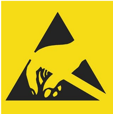
Figure 1.2: Symbol indicating ESD susceptibility, used to mark items that require controlled handling. Extracted from: [6]
