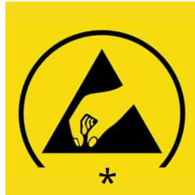
Figure 1.3: Symbol indicating an ESD protected handling area or protective equipment for controlled operation. Extracted from: [6]
