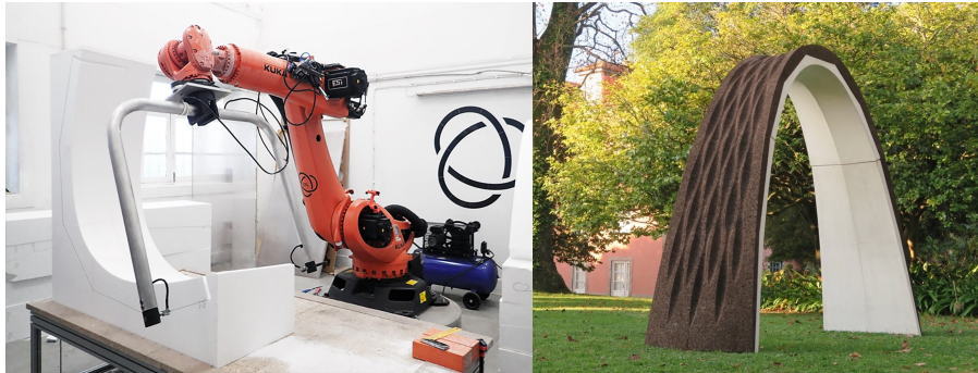
Figure 1. Previous research conducted by the authors involved the construction of the CorkCrete Arch prototype, which featured a combination of cork and GFRC panels, which derived from RHWC produced molds. Source: Sousa & Martins, 2016.
