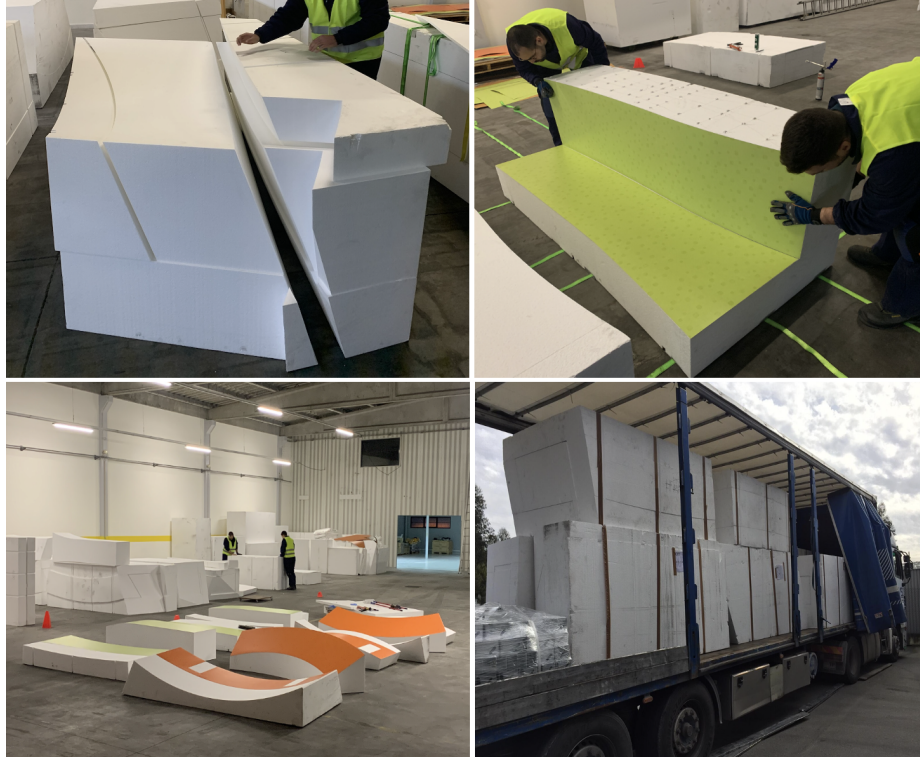
Figure 6. Cut molds before and after thermolaminated sheet placement and packaged transport. Source: authors.
