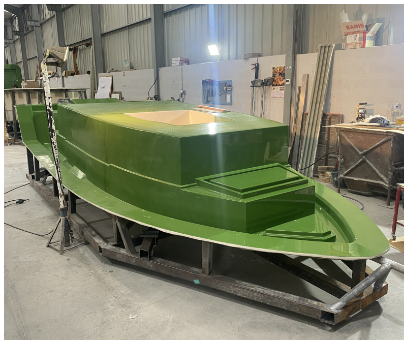
Figure 4.28: Mold of the deck of the Evolution 5.0 vessel.
