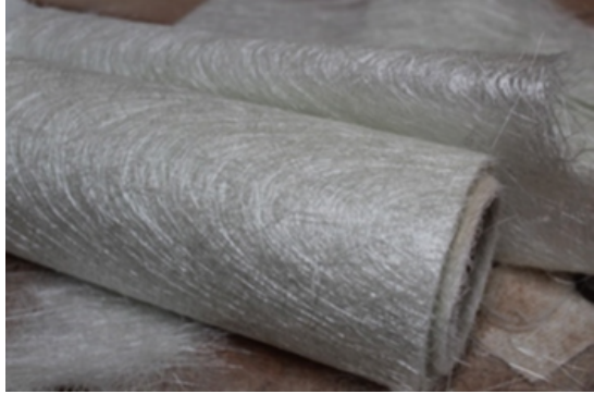
Figure 3.1: Dry fiber of chopped strand mat [48].
