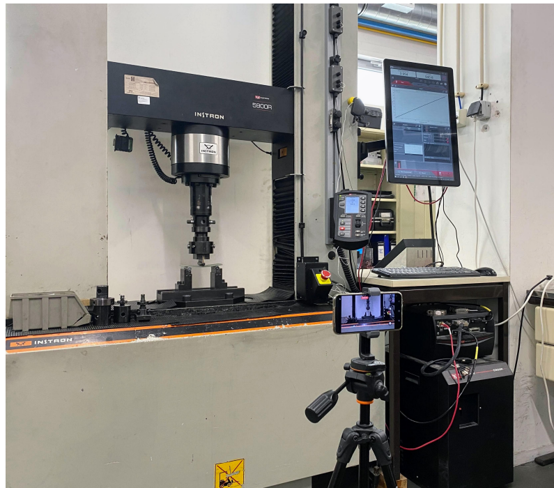
Figure 3.16: Global view of the setup used for the three-point bending tests.
