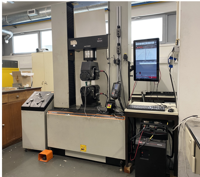
Figure 3.9: Global view of the setup for tensile tests; to be highlighted the hydraulic grips and their control equipment (on the left of the tensile machine), besides the computer numerical control of the tensile machine (on the right side).
