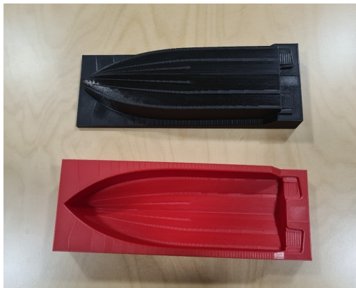
(a) 3D printing of the hull molds [47]
