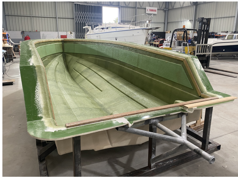
Figure 4.27: Mold of the hull of the Evolution 5.0 vessel.
