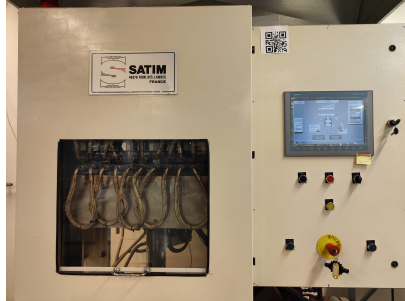
(a) Hot-press used for consolidation.
