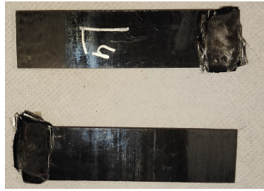
(a) Adhesive failure: clean debonding.
