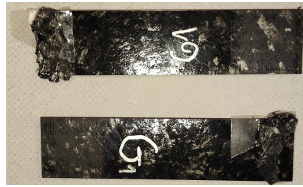
(c) Mixed-mode failure: torn ED film.
