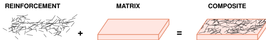
Figure 2.1: Schematic representation of a composite formation.
