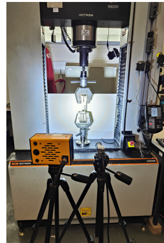
(b) Extended setup for DIC.
