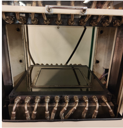
(c) Metallic frame used for moulding.
