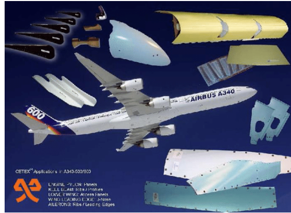
Figure 2.5: Application of PPS in the Airbus A340 [16].
