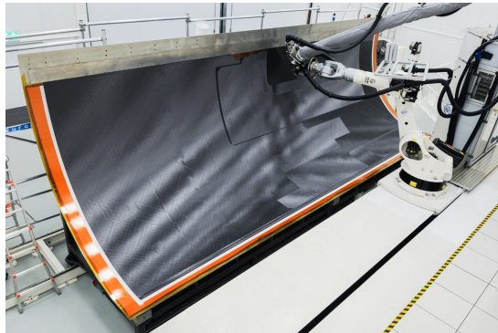
(a) Full 8-meter MFFD fuselage shell.
