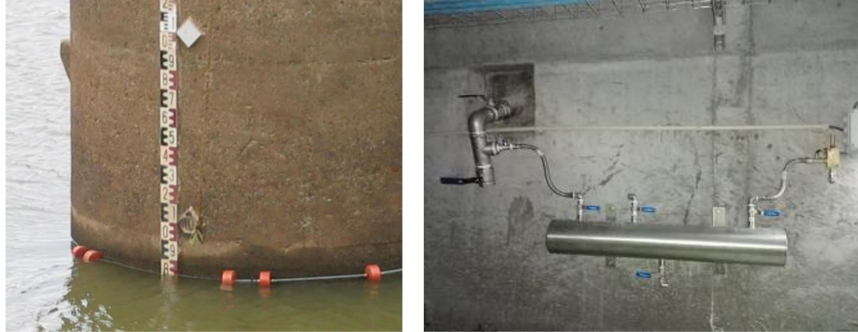
Figure 2.5: Limnimetric scale for manual water level measurement (left). Hydrostatic pressure sensor for automated water level measurement (right).
