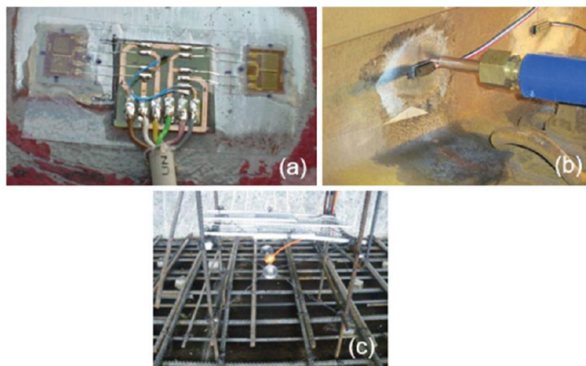
Figure 2.2: Strain gauges used in civil testing. a) resistance-based glued, b) resistance-based welded, c) embedding resistance strain gauge inside the concrete element. Adapted from (Borosc hek and Santos, 2020).
