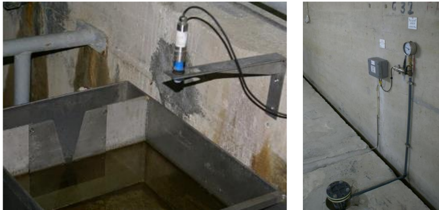
Figure 2.7: Measuring weir for discharge measurements to evaluate the amount of water that flows through the dam (left). Apparent part of a piezometer to measure the uplift pressure placed on the rock mass foundation (right).
