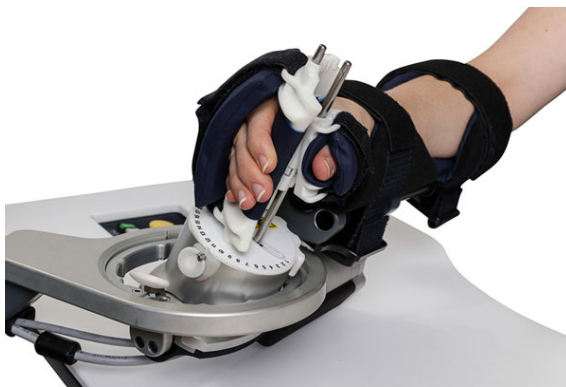
Figure 2.12: BIONIK's Arm/Hand end effector solution for upper limb rehabilitation [45]
