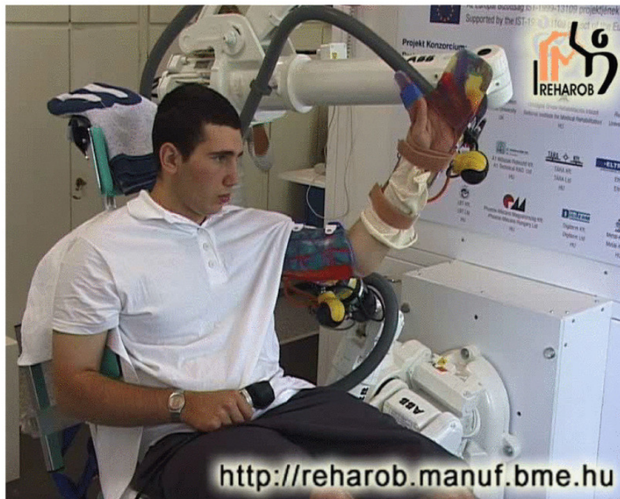
Figure 3.3: REHAROB Robotic rehabilitation system for upper limb motion therapy for the disabled [77]
