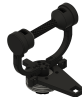
Figure 5.10: No load AK60 Motor test setup
