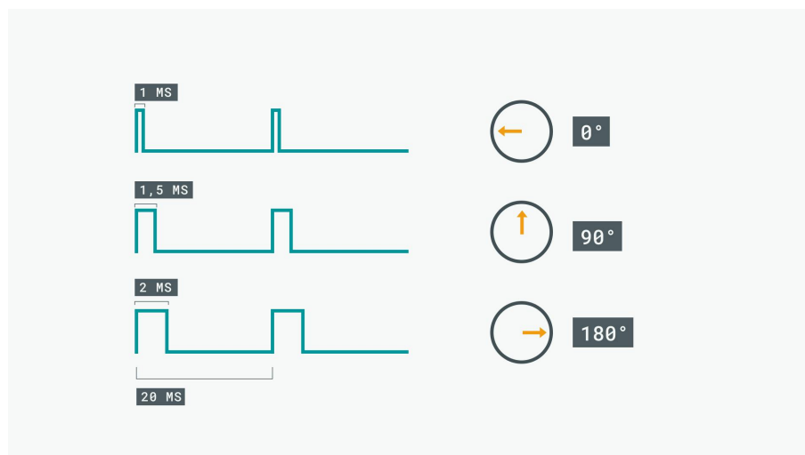
Figure 2.10: Servo motor positioning [13]
