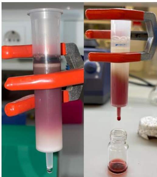
Figure 10. Molecule separation using a Sephadex G-25 column according to their relative size, where small molecules (like sodium dithionite) are efficiently separated from high-molecular-weight molecules of interest, hemoglobin in this case.
