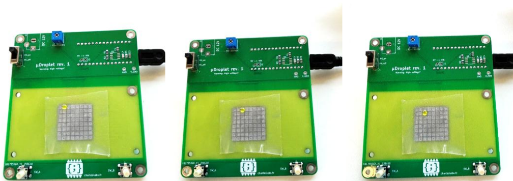
Figure A6 Droplet progression on a microfluidic platform under sequential electrode selection.
