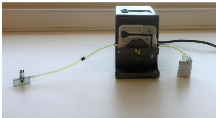
Figure 24 3D printing microfluidic module designed for incubation and calibration of electrochemical sensors.
