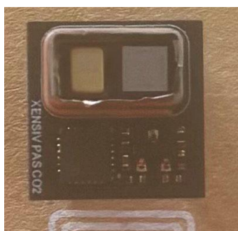
Figure A3 Visualization of transduction components with an infrared source (square-shaped component) on the right and a MEMS microphone (yellow rectangular component) on the left.
