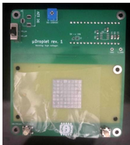
Figure A5 Electrode Matrix on \mu Droplet replica PCB (8x8).
