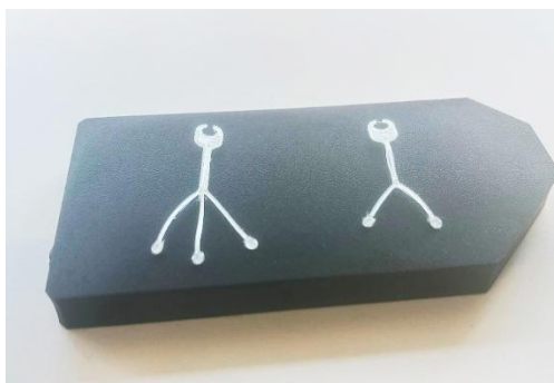
Figure A20 PVA molds for microfluidic channels produced using conventional 3D printing [129].
