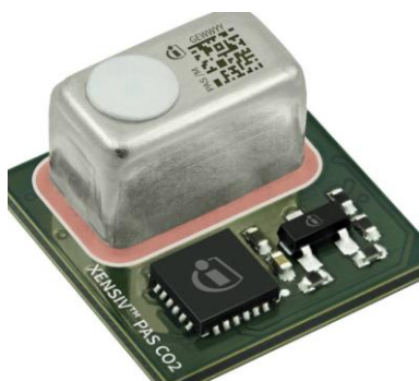
Figure A2 XENSIVPASCO2 photoacoustic sensor. Below the red circle, a hole serves as the access point for CO 2 gas after it is released from the degradation cell of the Fenton reaction. It is also important to highlight the presence of a complex signal amplification circuit integrated into the PCB associated with the sensor.
