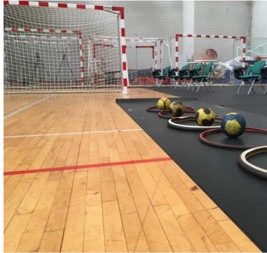
Figure 12. The setup for the data collection with the 4 balls with different weights and the radar behind the goal
