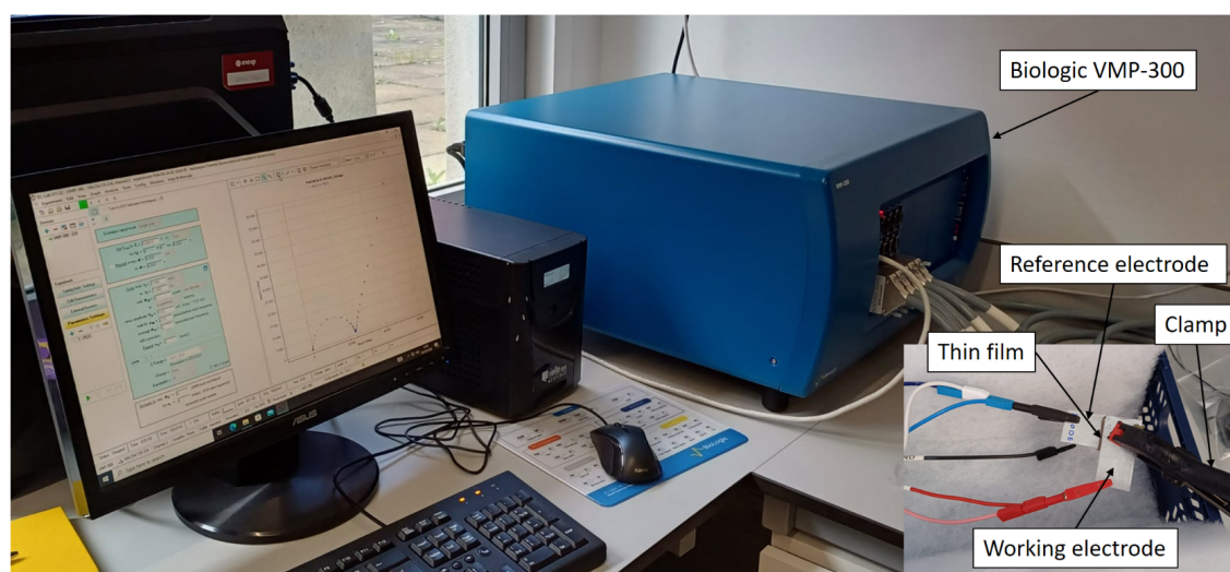
Figure 7.6: Measuring the PEIS of thin films using Biologic VMP-300.
