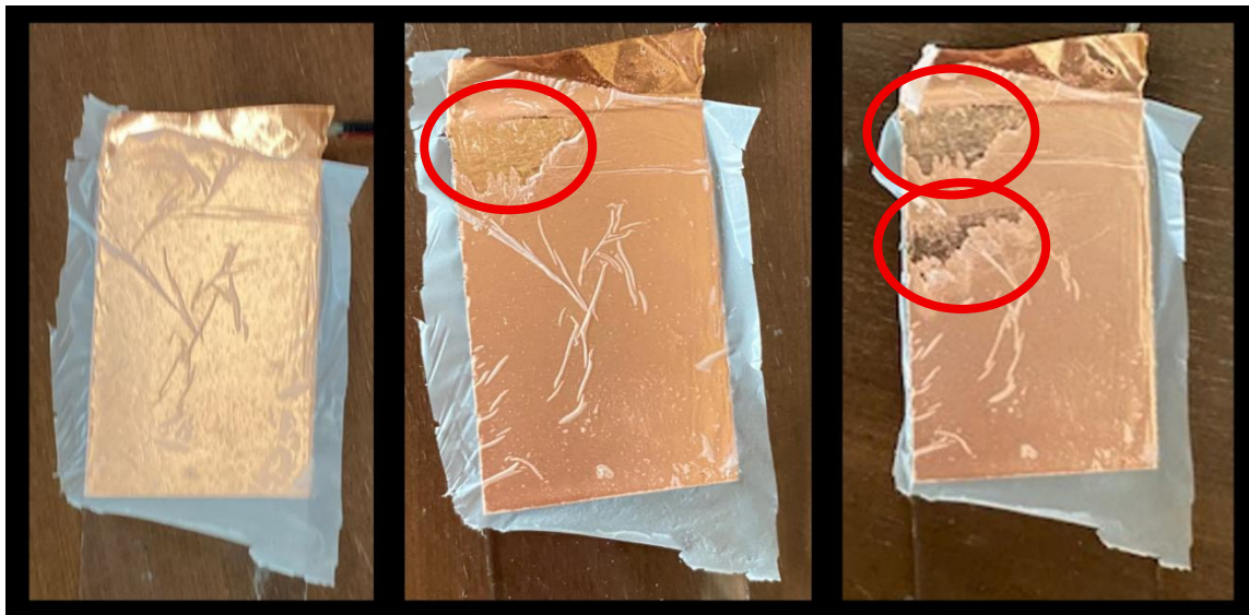
Figure 26 – PDVF fibre samples before (left) and after (centre, right) use. Exposed copper highlighted
