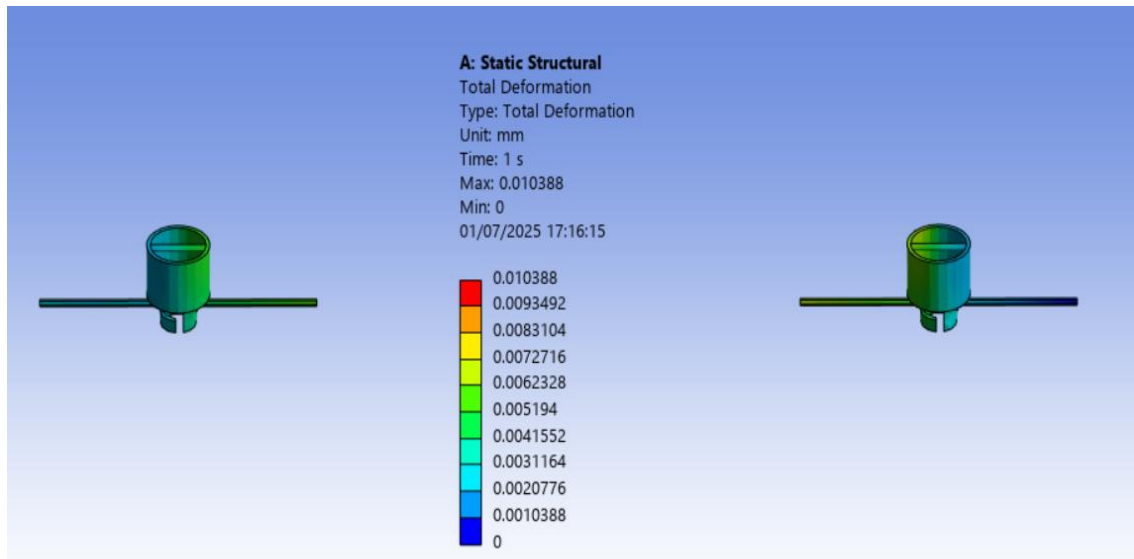
Fig. 37 - Localised deformation in the connector and embedded rebars.
