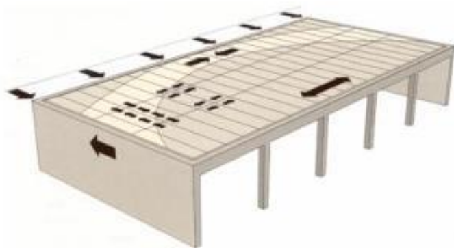
Fig. 5 - Development of forces in a diaphragm (Joostdevree, 2024)
