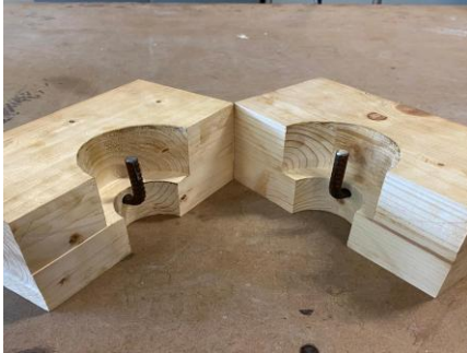
Fig. 21 - Upward-bent rebar + timber block.
