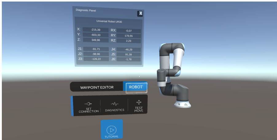
Figure 5.8: Diagnostics panel of the AR interface, showing real-time feedback from the UR30. The panel displays the Cartesian position and orientation of the TCP (X, Y, Z, RX, RY, RZ), as well as the six joint angles (J1–J6). This transparency allows the operator to validate the robot’s current state and verify that data streaming from port 30013 is functioning correctly.
