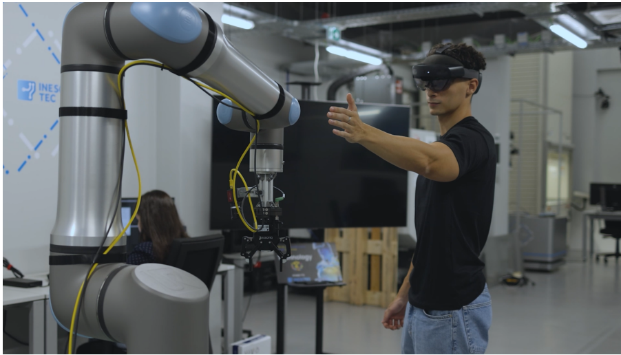
Figure 5.14: Protective stop triggered during system testing when a user places the hand close to a collider.
