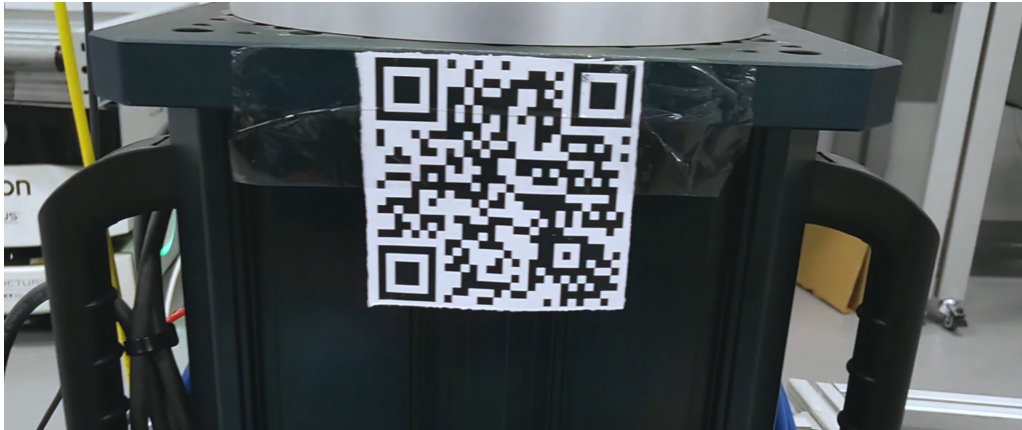
Figure 5.15: QR-based calibration as seen through the AR glasses. The system detects the pose of the marker in the world frame ( {}^W T_M ) and combines it with a fixed offset to the robot base ( {}^M T_B ), resulting in the robot base pose in world coordinates ( {}^W T_B ).
