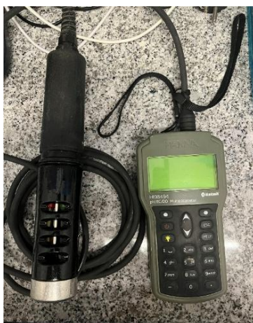
Figure 26 - Multiparameter probe for measuring water parameters (Author: Maria Castelo).
