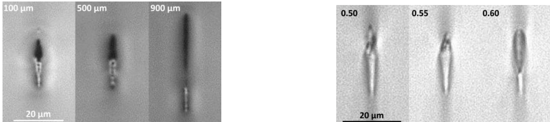
Figure 2.3: Cross-section view of waveguides inscribed in Suprasil 1. Pulse energy and writing velocity fixed at 200 nJ and 100 \mu s^{-1} . left: Dependence on written structures with inscription depth; right: Dependence on written structures with NA [2]
