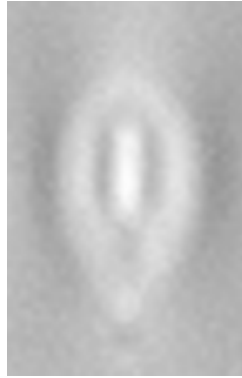
Figure 4.1: Transmission mode optical microscope image of the cross-section of a waveguide produced on an EAGLE2000 glass substrate.
