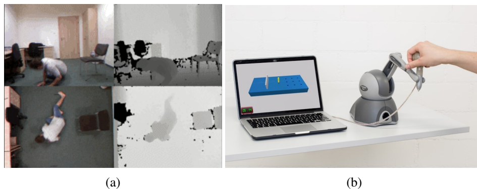
Figure 2.8: Example data from two healthcare and rehabilitation datasets: (a) UR Fall Detection: sample frames showing a fall event captured using RGB and depth cameras (Kwolek and Kepski (2014)). (b) U-Limb: representation of multimodal data acquisition during upper limb movement task, including kinematic measurements and physiological signals (Averta et al. (2021)).
