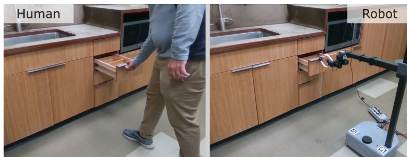
Figure 2.15: Example of a drawer-opening task: on the left, the action is performed by a human; on the right, the same action is executed by a robot through imitation. Source: Bahl et al. (2022)
