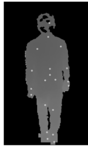
Figure 4.21: Depth-Based Gait Dataset: sample depth-map frame with overlaid skeletal joints, illustrating joint locations.
