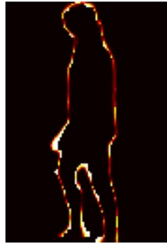
Figure 5.10: Error Map visualization of interpolation results. Each pixel value represents the absolute reconstruction error between the predicted and ground-truth silhouettes, encoded using the “hot” colormap (black = perfect agreement, yellow-white = increasing error).
