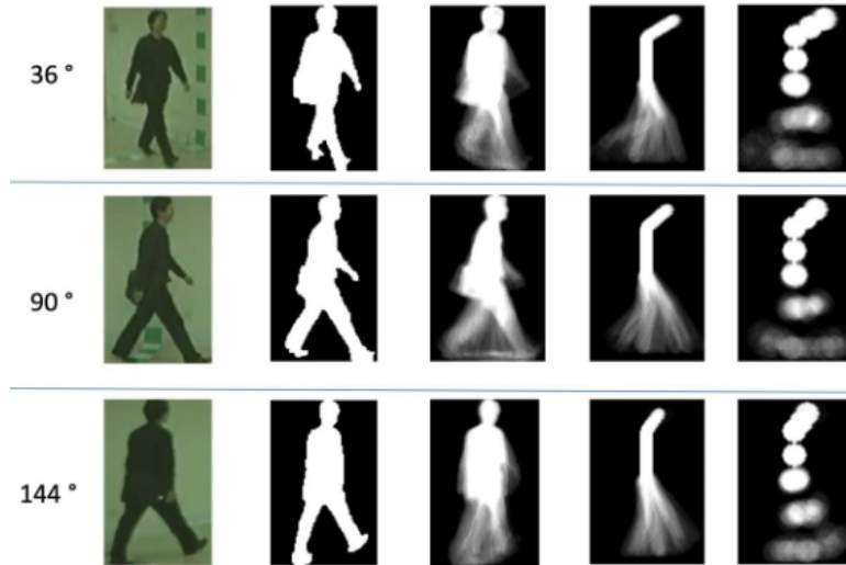
Figure 6.6: Comparison of gait representations from three viewpoints. For each perspective, the sequence illustrates the RGB reference image, the corresponding silhouette, the Gait Energy Image (GEI), and the two proposed GSI variants: line-based and joint-based representations.
