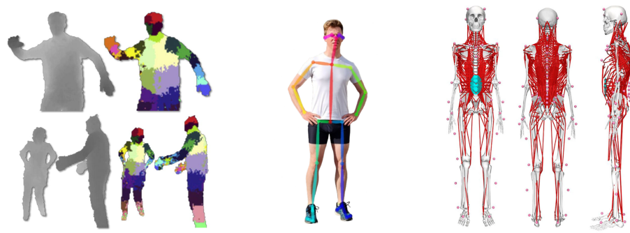
Figure 2.5: Examples of technologies and models used in human motion analysis: (a) depth map generated by a depth sensor; (b) 2D skeletal tracking overlaid on an RGB image of a human subject; (c) various biomechanical models representing the human body for motion analysis.
