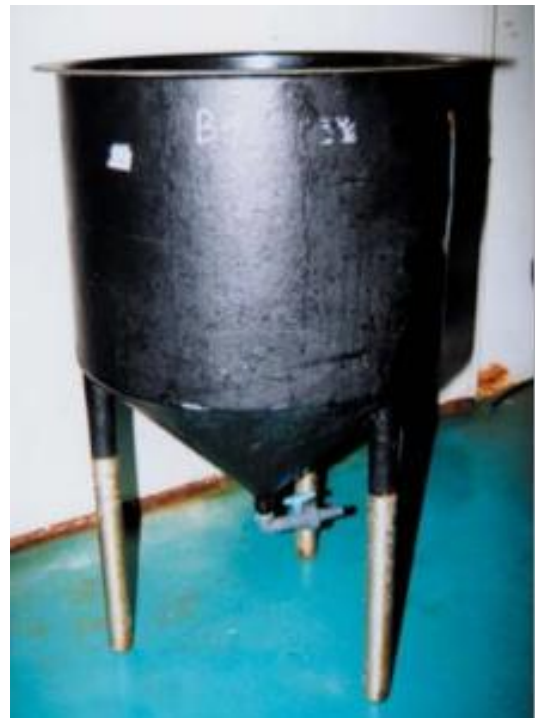
Fig. 11– Fiberglass cylindroconical tank used for eggs
