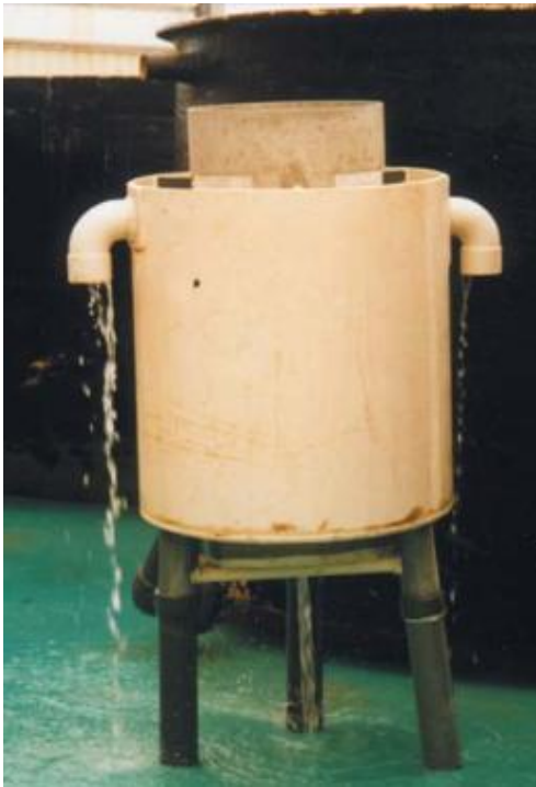
Fig. 10– Overflow collector (Moretti et al., 1999)
