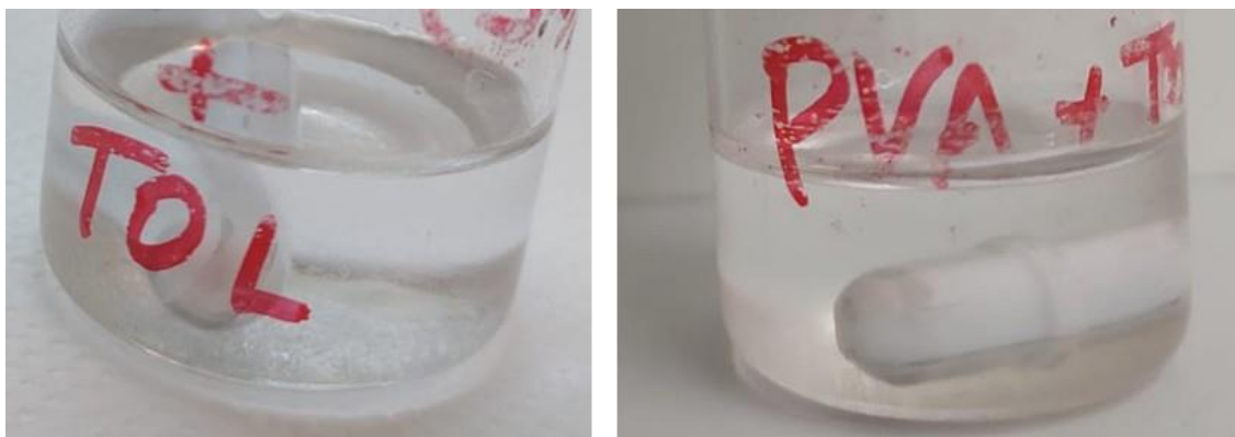
Figure 12: Results from solubility tests performed with PVA in toluene. (Left) After 24 hours stirring at room temperature, PVA particles are visible, deposited on the bottom of the flask; (Right) After 24 hours stirring at 40 °C a homogeneous solution is obtained.
