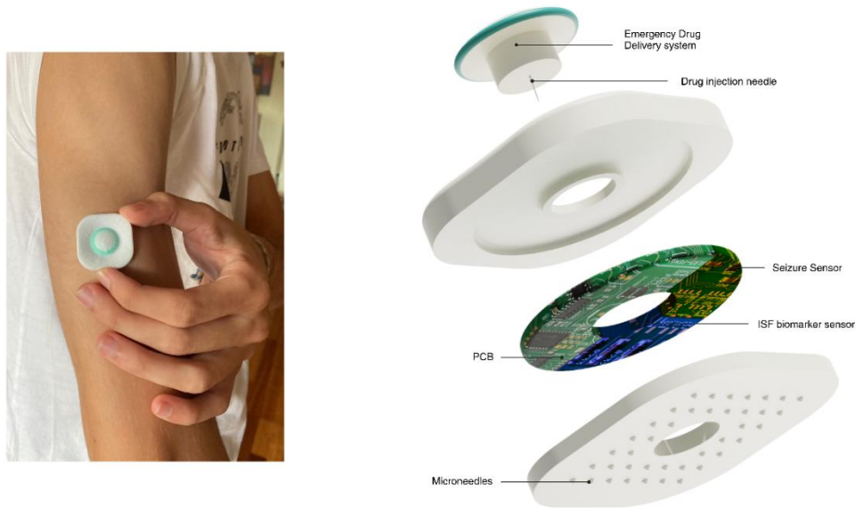
Figure 4.1 Overview of the AI-CLD system, consisting of a continuous seizure detection sensor, a SUDEP biomarker sensor, a processor, and an emergency drug delivery actuator processor immediately triggers the actuator to deliver a SUDEP preventing intervention, e.g., an appropriate dose of a SUDEP preventing medication ( Figure 4.2 – action 5 ). Simultaneously, the AI-CLD communicates with a mobile device ( Figure 4.2 – action 6 ) to
