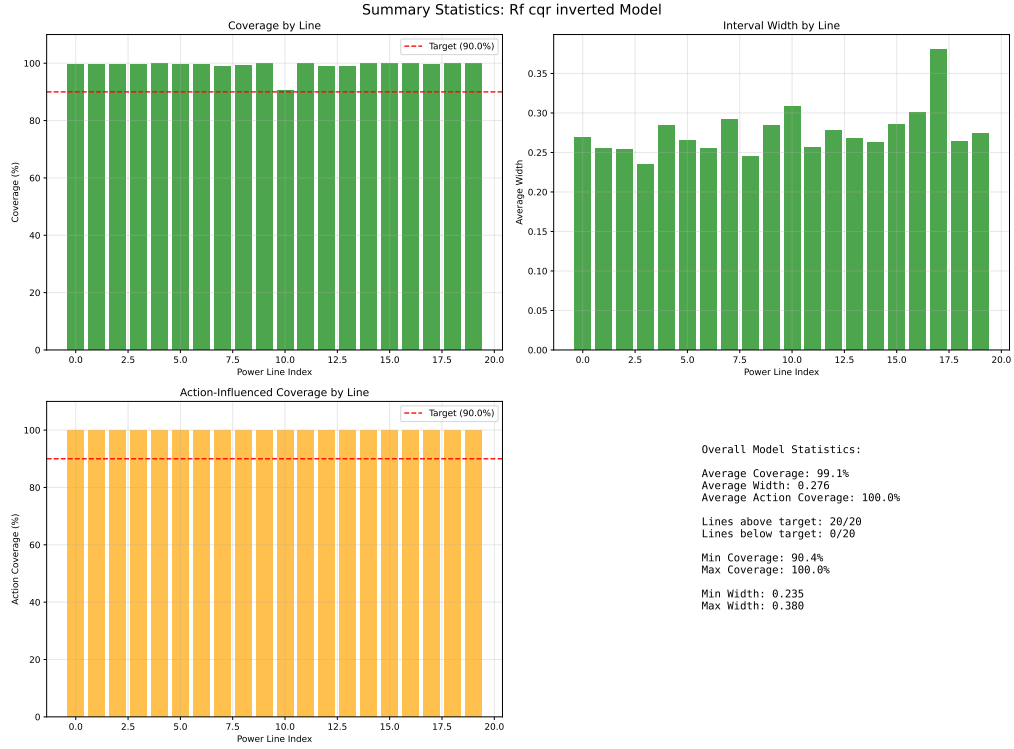
Figure A.32: Case Study 2 Inverted RB-CQR with Random Forests: Conservative over-performance in almost all lines, with clear efficiency disadvantages.
