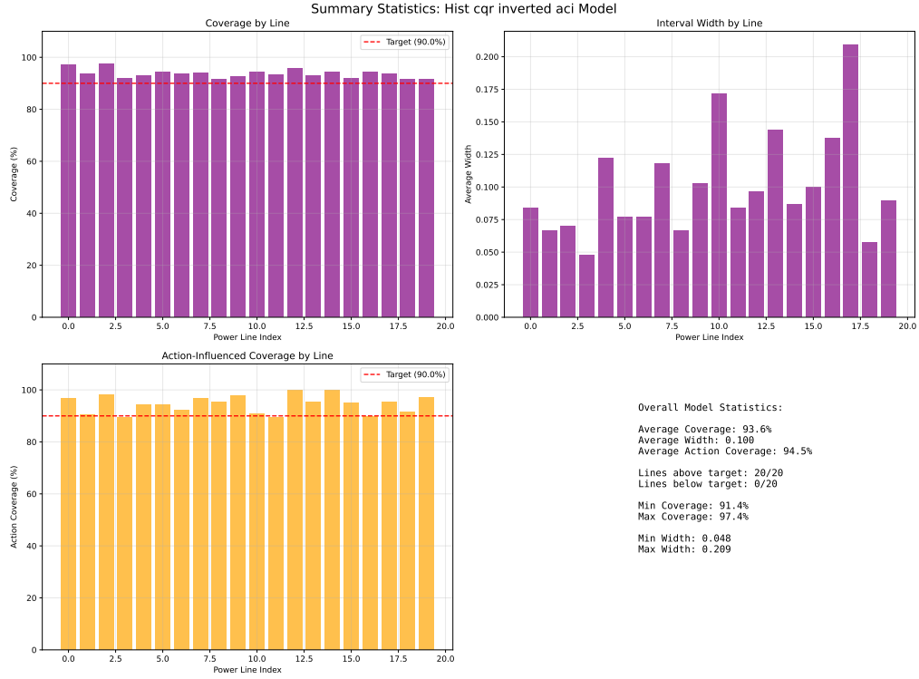
Figure A.18: Case Study 1 Inverted RB-CQR with Histogram Gradient Boosting and ACI update rule: The best Inverted RB-CQR configuration, showing still excellent coverage with superior width efficiency, when compared to the other backends.
