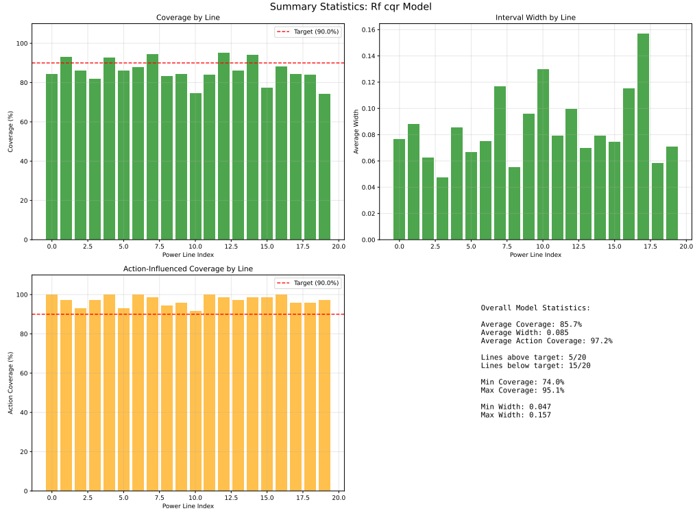
Figure A.27: Case Study 2 RB-CQR with Random Forests: Summary statistics of the best-performing RB-CQR backend, without the ACI update rule. There are some lines that are far from the coverage objective.
