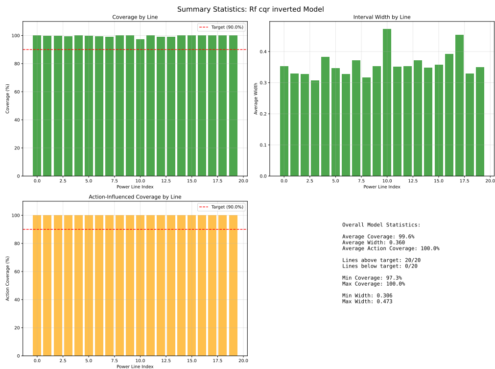
Figure A.47: Case Study 3 Inverted RB-CQR with Random Forests: Excessive conservatism demonstration, showing that although the coverage is met, the efficiency is too reduced.
