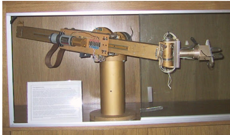
(a) Stanford arm with six degrees of freedom, designed at Stanford University by Victor Scheinman in 1969 [9].
