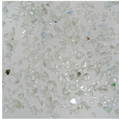
(a) Flint cullet: composed mainly of transparent glass fragments.
