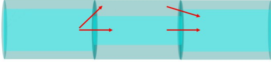
Figure 2.11: Representation of a fiber Mach-Zehnder interferometer, adapted from [66].
