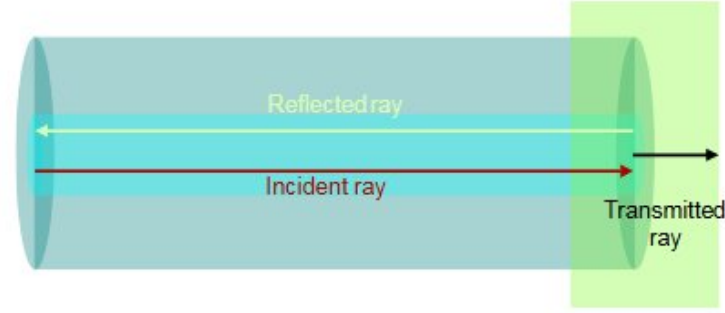
Figure 3.2: Representation of light propagation when the cleaved tip is in contact with the external medium.
