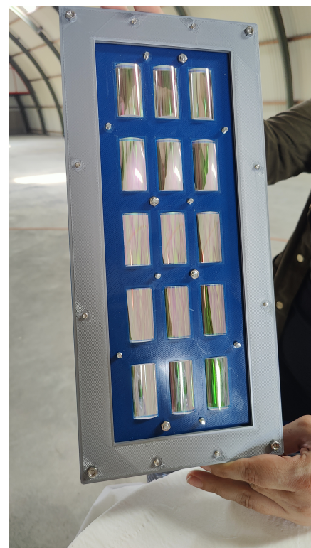
Figure 3.16: (a) Schematic drawing, and (b) picture of the spherical and cylindrical lens matrices.
