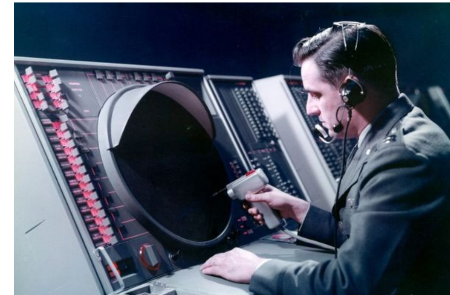
Figura 1. Trabajador usando el SAGE (Semi-Automatic Ground Environment). Fuente: Computer History Museum
