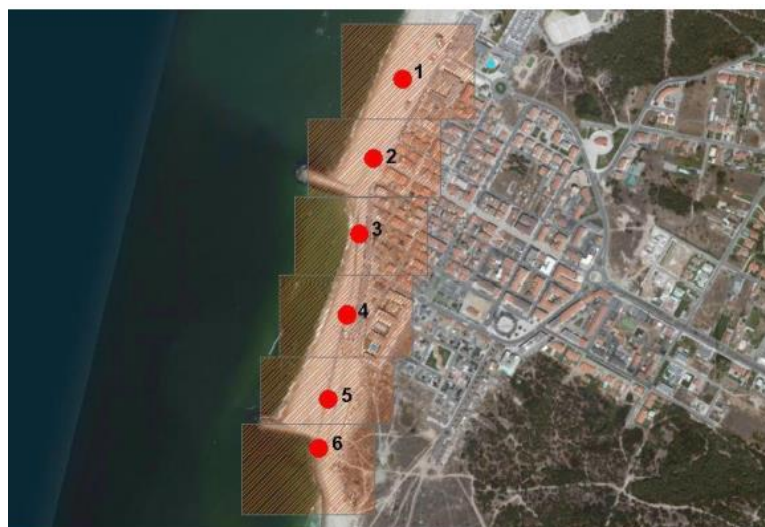
Figure 3.13 - Zones of influence of each structure for the risk calculation (ArcMap 10). Adapted from Martins, 2016.
