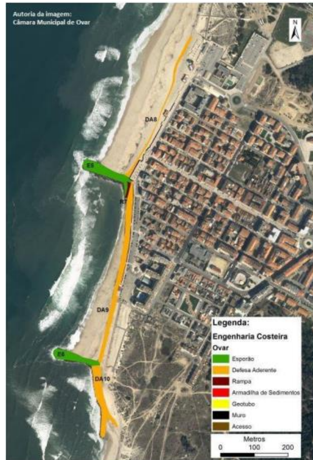
Figure 3.2 - Coastal defense works at Furadouro Beach (Câmara Municipal de Ovar, 2012, adapted from Marques, 2021).
