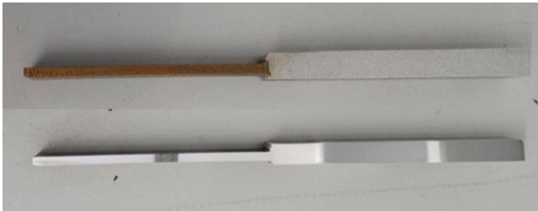
Figure 19: Before (above) and after (below) polishing treatment
