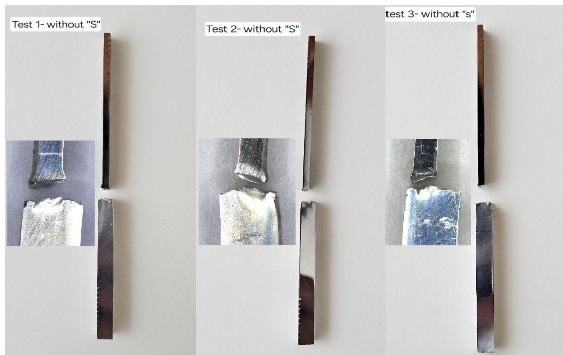
Figure 29: Tensile test, failure location (IMC) in test 1, 2 and 3- without "S"
