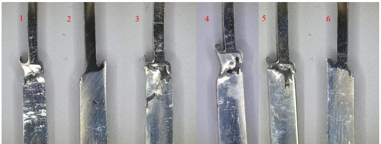
Figure 35: Failure modes observed in “with S-shape” profiled joints after fatigue testing
