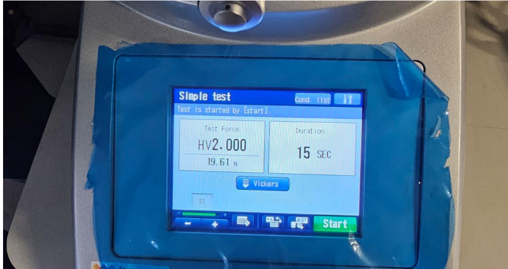
Figure 24: Control panel of the Vickers microhardness tester showing the test parameters used.
