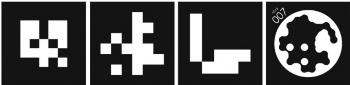
Figure 2.1: Fiducial markers examples, from [9]. From left to right, ARTAg, AprilTag, ArUco and STag
